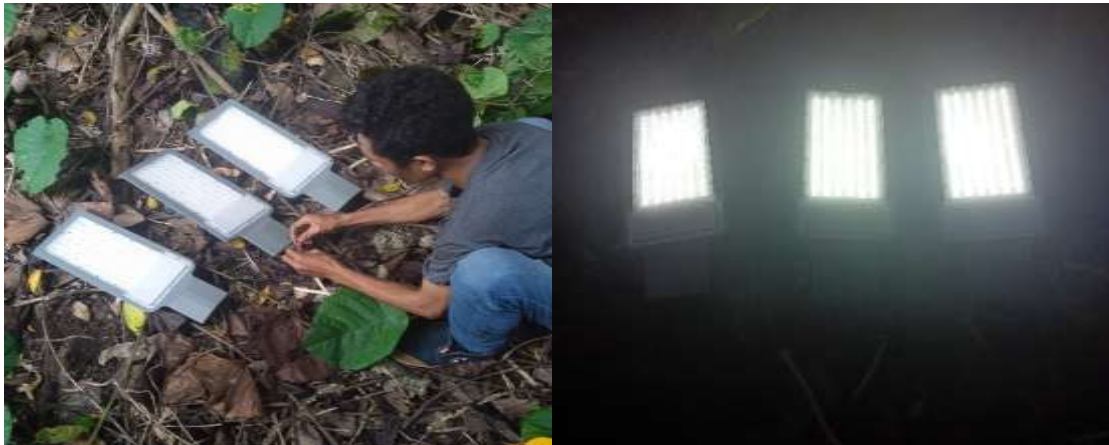
Gambar 6. . Pengujian Lampu LED 100 Watt
