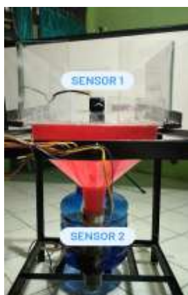
Gambar 8. Posisi sensor waterflow
